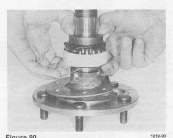
With tape still wrapped around the ring, push seal up until it contacts the rib ring. This will force the grease up through the rollers.
