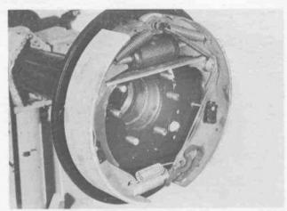
Assemble backing plate bolts and backing plate assembly.
