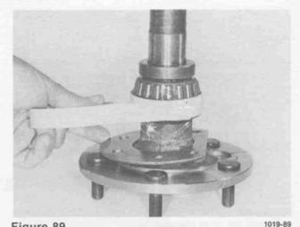
After the cavity is full of grease, wrap tape completely around the rib ring and seal as shown to enclose the cavity.
